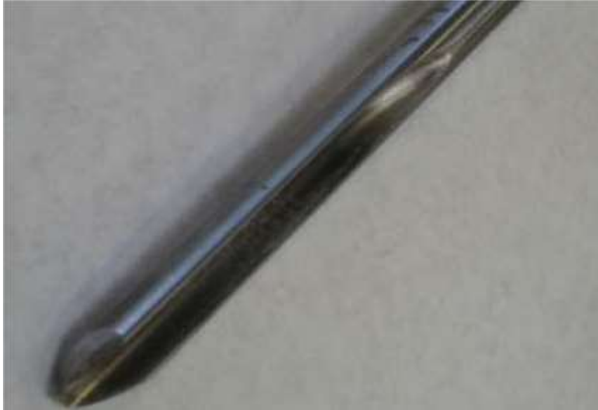
c. Bowl gouge —shallow fluted spindle gouge or detail gouge.
